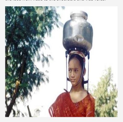
The innovation is a boon to women who need to carry loads for more than ten to twenty miles, from wells and springs to their households. The device has a headrest where the load will be stationed, along with two extending support rods that originate from the sides of the head rest. The weight is effortlessly transferred to the shoulders. When Khimjibhai developed the concept, he did not make much progress since his neighbors and friends did not take the idea seriously.
