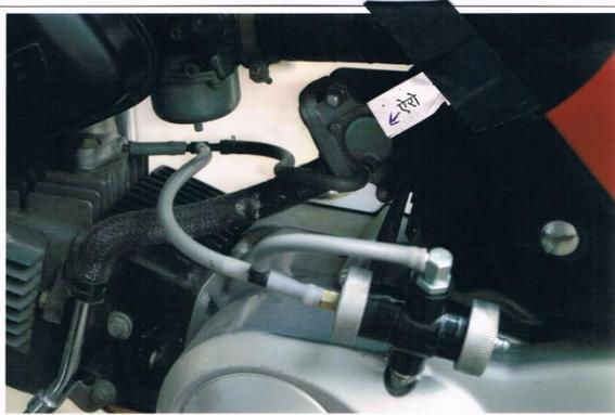
The device sucks in and stores an extra layer of air-fuel mixture, which is released back into the engine. The timing of such release is strategic and is introduced just ahead of
